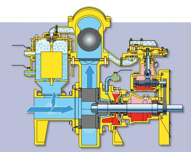
After starting the unit, the vacuum pump starts priming air out of the suction line. A non-return valve shuts off the discharge side. As soon as the pump is primed, the float closes the vacuum pump connection and the centrifugal pump starts pumping liquid.
